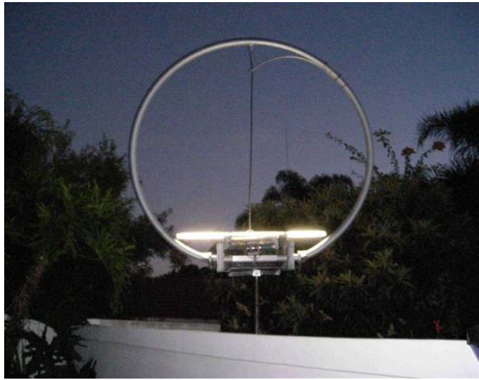
This striking shot is of Ed ZS6UT's magnetic loop (described in WATTS Aug 2003). Here an incandescent tube was placed close to the feedpoint and was greatly excited due to the high voltage field running 200w PEP on 80m. Ed says you can actually read the light semaphore effect.
